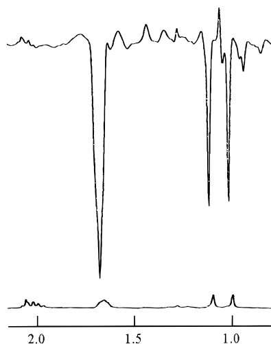
Figure 1. 1 H NMR spectra (80 MHz) of acetone- d 6 solutions containing 30 mM cis -chrysanthemol ( cis - 2 ) and 5 mM chloranil in the dark (bottom) and during UV irradiation (top). Only the resonances of the non-equivalent pairs of methyl groups (allylic, ~1.6 ppm; cyclopropane, ~1.1, 1.0 ppm) show significant polarization.
